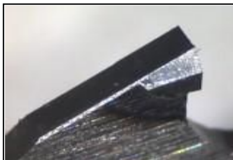
Tooth from a 3860 Multi-Chip Unset Carbide Tipped bandsaw blade.
